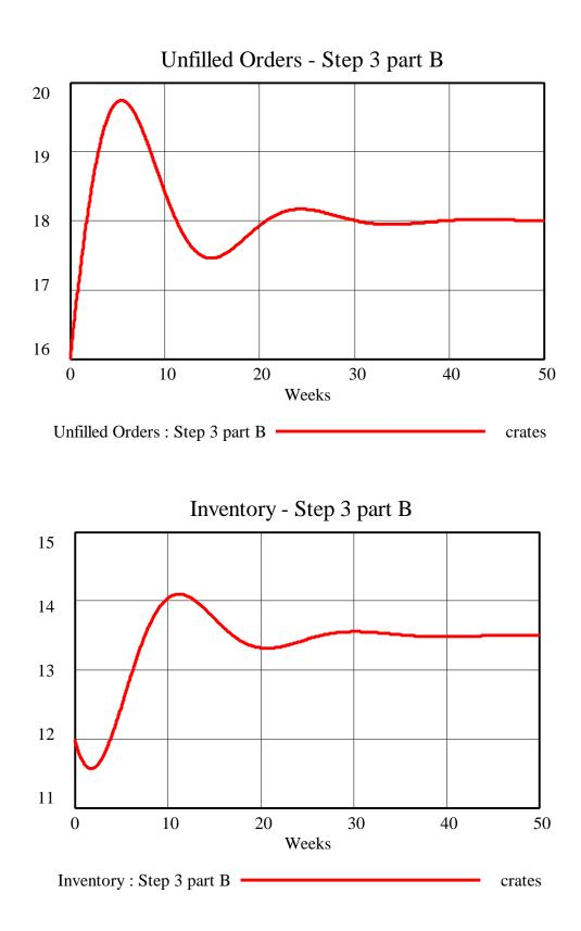
This scenario mimics the scenario from Step 1 part B, before pipeline ordering was added to the model. A "PIPELINE RECOGNITION FACTOR" of 0 means that Jim does not take into account any of the orders that are in the pipeline when he is making new orders.
