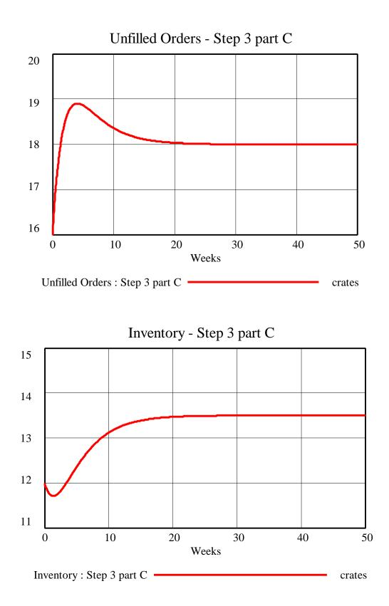
This scenario mimics the scenario from Step 2 part D, after pipeline ordering was added to the model. A "PIPELINE RECOGNITION FACTOR" of 1 means that Jim takes into account all of the orders that are in the pipeline when he is making new orders.
