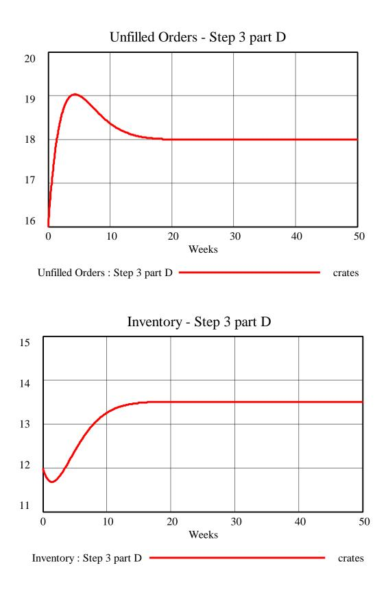
Even though in this scenario Jim recognizes only 75% of the orders in the pipeline, the behavior is almost as stable as if he took into account the entire pipeline. The higher the "PIPELINE RECOGNITION FACTOR," the more stable the system behavior.
