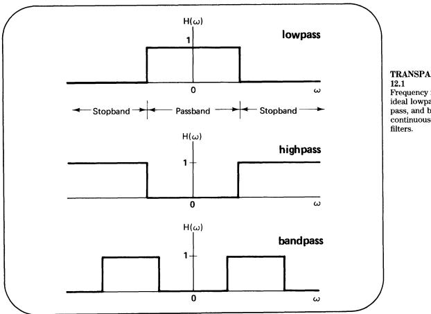
TRANSPARENCY 12.1 Frequency response of ideal lowpass, highpass, and bandpass continuous-time filters. TRANSPARENCY 12.2 Frequency response of ideal lowpass, highpass, and bandpass discrete-time filters.
