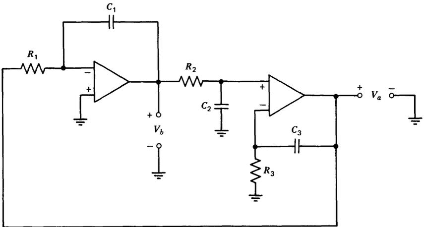
**Figure 12.2** Quadrature oscillator.
