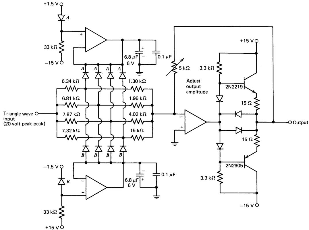
**Figure 12.35** Sine-wave shaper.
