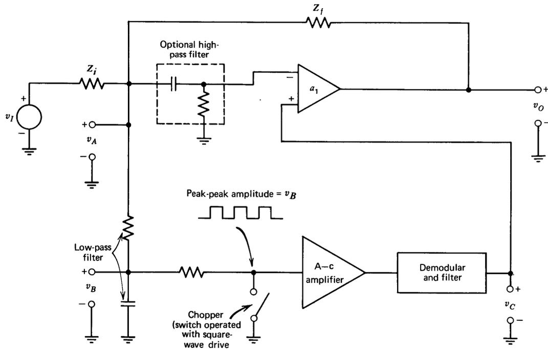
Figure 12.21 Chopper-stabilized amplifier.
