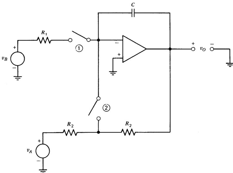
Figure 12.17 Three-mode integrator.
