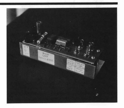
This lecture continues examples of describing-function analysis. The method is used to predict the operation of an oscillator formed by combining an integrator with a Schmitt trigger. Reasonable agreement with the exact solution is obtained even though the conditions assumed for describing-function analysis are not particularly well satisfied by this system.
